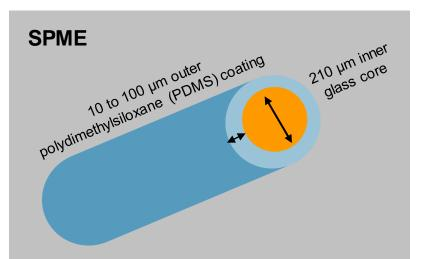
SPME figure from: Burgess, R.M., 2013. *Passive Sampling for Measuring Freely Dissolved Contaminants in Sediments: Concepts and Principles*. Training Slides from 23rd Annual NAPRM Training. U.S. Environmental Protection Agency ORD NHEERL. Available at: https://clu-in.org/conf/tio/Porewater2\_111914/resource.cfm.
