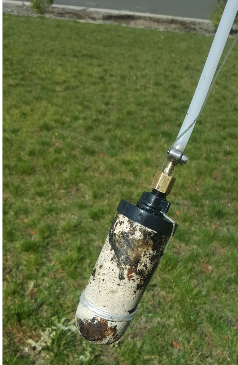
Intake mode (after sampling groundwater below light nonaqueous phase liquid in well)
