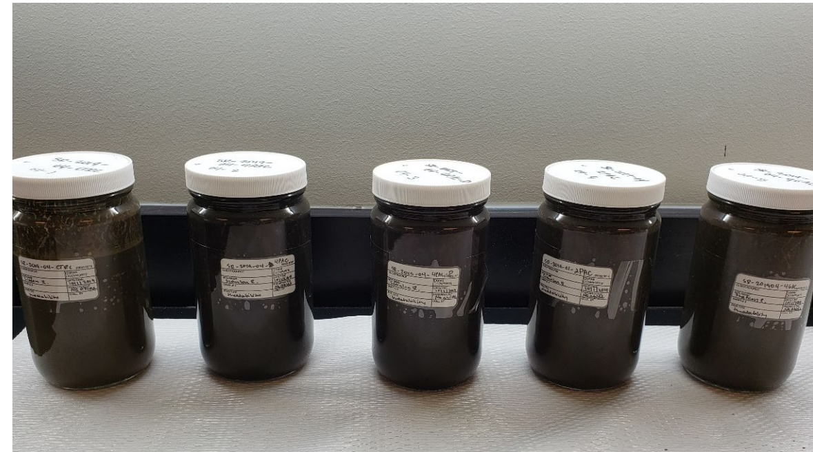
Bench-scale treatability study mesocosms
