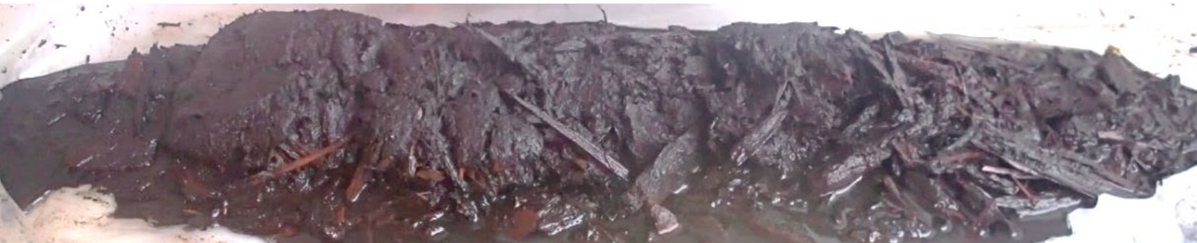
Core sample showing thickness of woody layer
